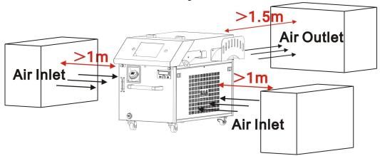
4. Determine the direction of the pipeline layout according to the water inlet and outlet of the chiller, and ensure that the waterway is clean and free of impurities, so as to prevent impurities from entering the waterway and causing blockage or pump failure.
